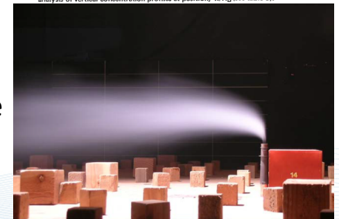
Figure 10. Vertical concentration profiles for isolated stack. In this and following legends, H_b/H_b identifies the presumed effective stack height as determined from analysis of vertical concentration profiles at position, x/H_b (see table 3).
